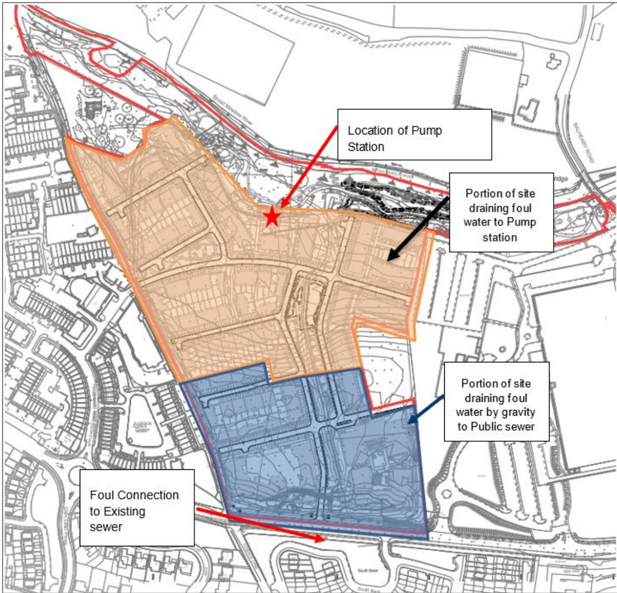
Figure 5.4 Indicative location of the pump station
